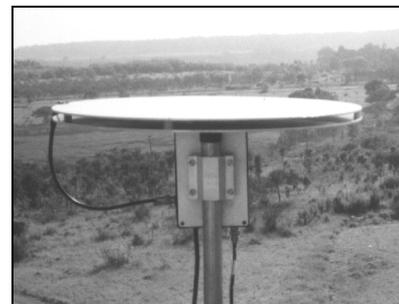
Figure 2 – Plate antenna
