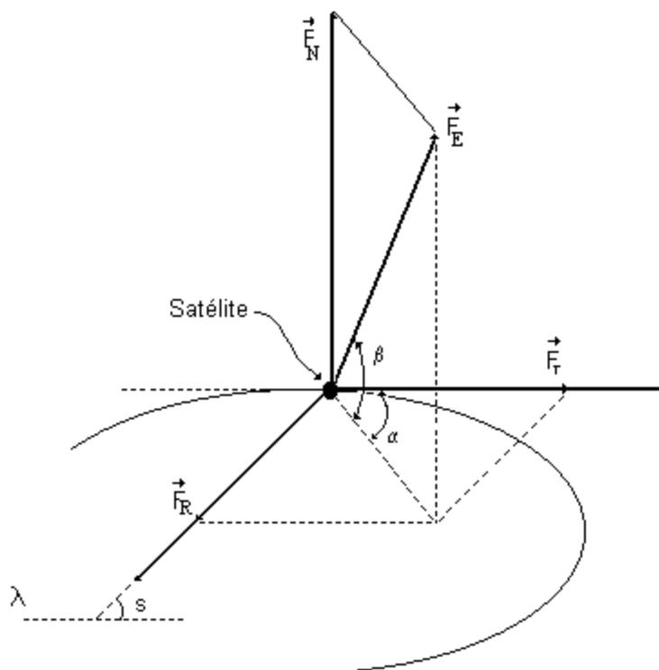
**Fig. 1 – The thrust vector applied to the satellite**
