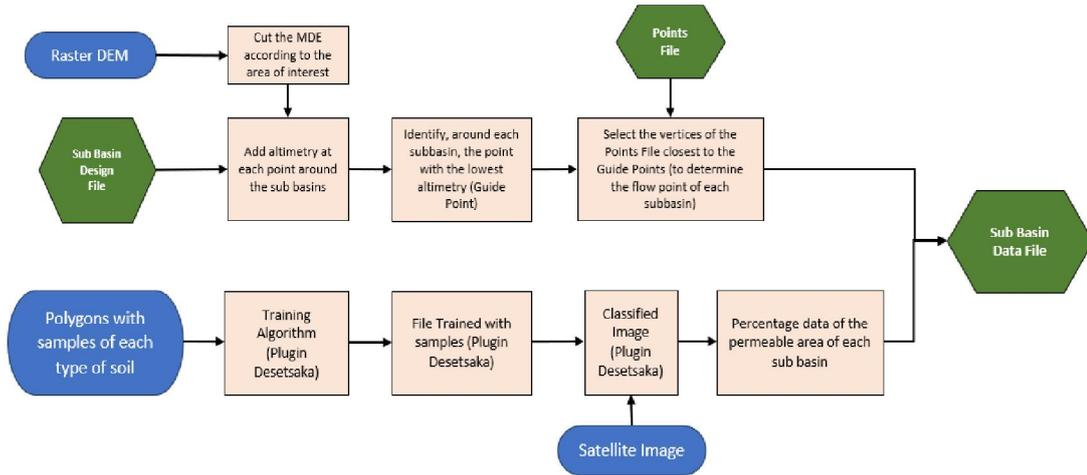
Figure 4 - Process diagram for generating the Sub-Basin Data File
