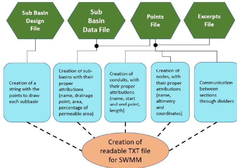
Figure 5 - Process diagram for generating the TXT file
