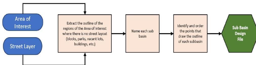
**Figure 3 - Diagram of the sub-basin generation process**
