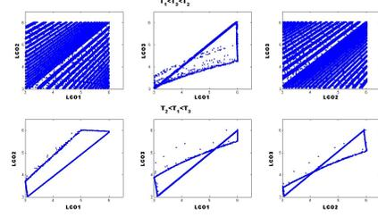
**Figure 2 – Trajectories in phase space for 3 LCOs when a MI coupling is established between them and differents detuning are used.**
