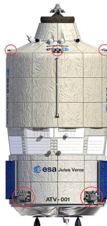
Figure 2.5 - ATV's reaction control system.
