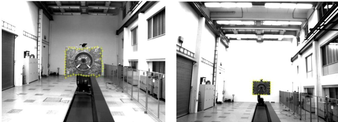
Figure 6.13 - Tracking edges of the target mock-up at 10 m (left) and 20 m (right).
