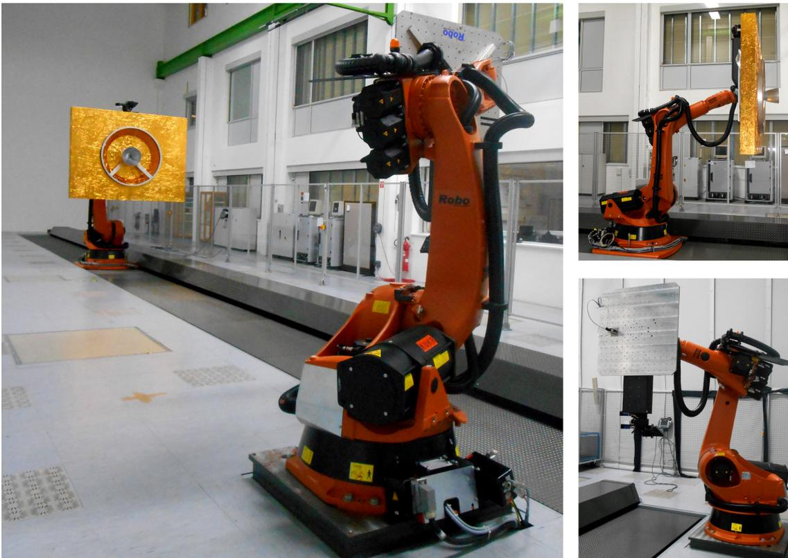
Figure 6.1 - The robots of the European Proximity Operations Simulator (EPOS).
