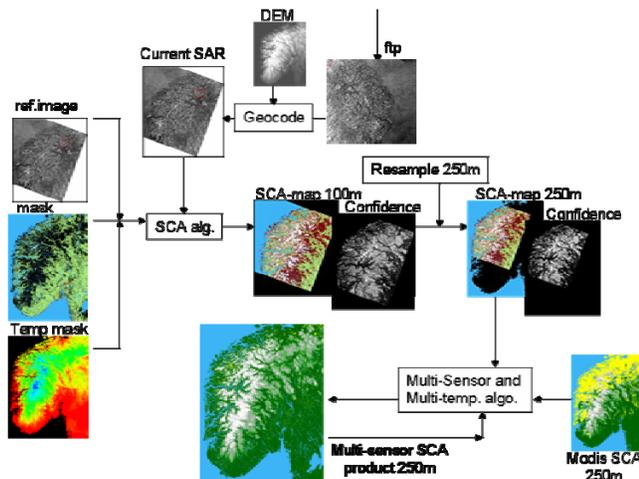
**Figure 1.** Schematic view of the SAR based snow cover area processing line. For snow cover area detection it is then combine with a MODIS snow cover in a multi-sensor product.
