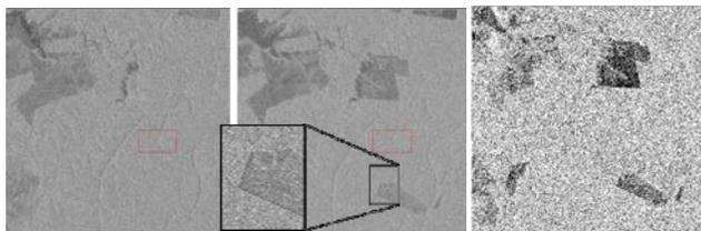
**Figure 2.** Envisat ASAR IMS sub-scenes from 24 Jul 2004 (left) and 13 Aug 2005 (center) and the thresholding result at  $-2.5\text{dB}$  of a simple subtraction (right) of the two scenes. The enlargement (black frame) shows SAR shadow (west) and corner reflector effects (east) of the trees on the border of the deforestation field. Images © ESA
