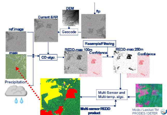
**Figure 3.** Schematic view of a possible new SAR based rainforest monitoring system that can complement existing operational optical monitoring systems. In the possible final result, old and new deforestation areas are yellow and red, respectively.
