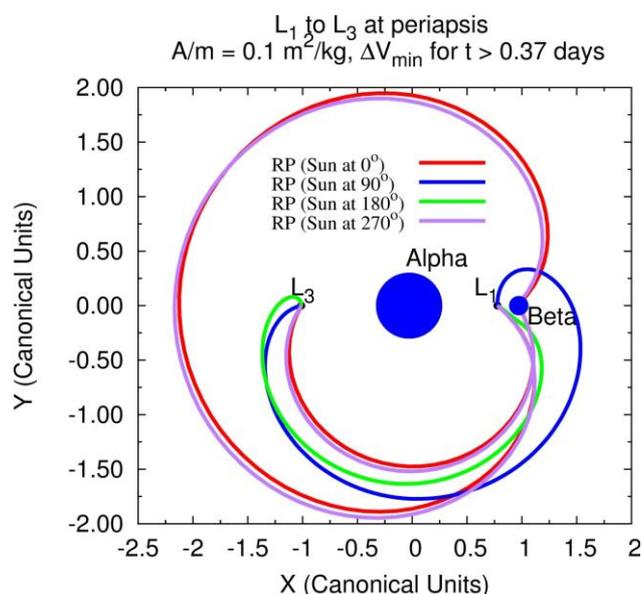
**Figure 1.** Trajectories between the Lagrange points of the asteroid 1996FG<sub>3</sub> considering the radiation pressure.
