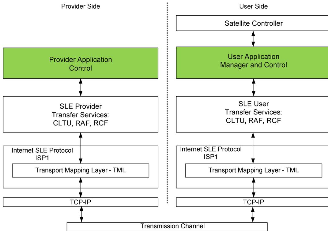
Figure 8. Architecture Model based on ISP1
