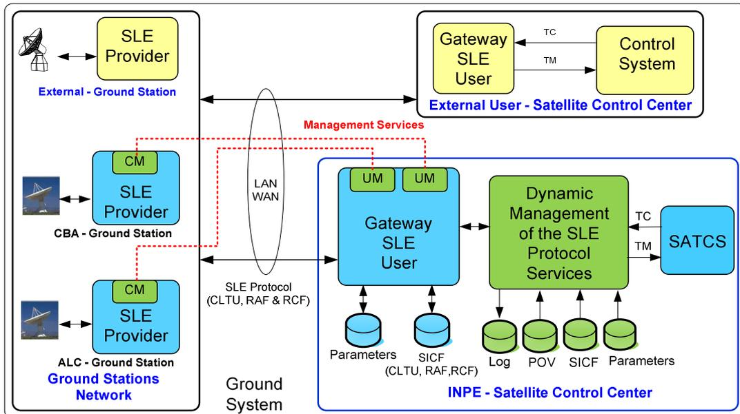
Figure 9. Environment for satellite operation with the dynamic management of the SLE protocol services
