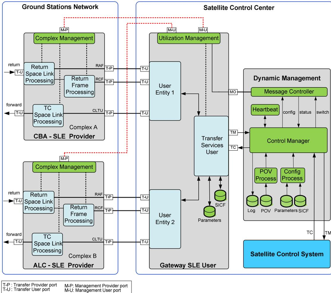
Figure 10. Architecture for Dynamic Management of the SLE Protocol Services
