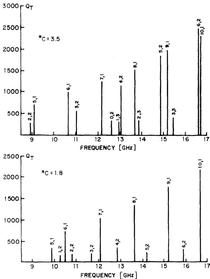
Fig. 4 Frequency spectrum for fundamental TE modes for the (a) 3.5-design and (b) 1.8-design  $C$  coaxial cavities
