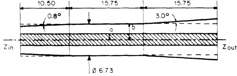
Fig. 1 Schematic diagram of the coaxial resonator (dimensions in cm)
