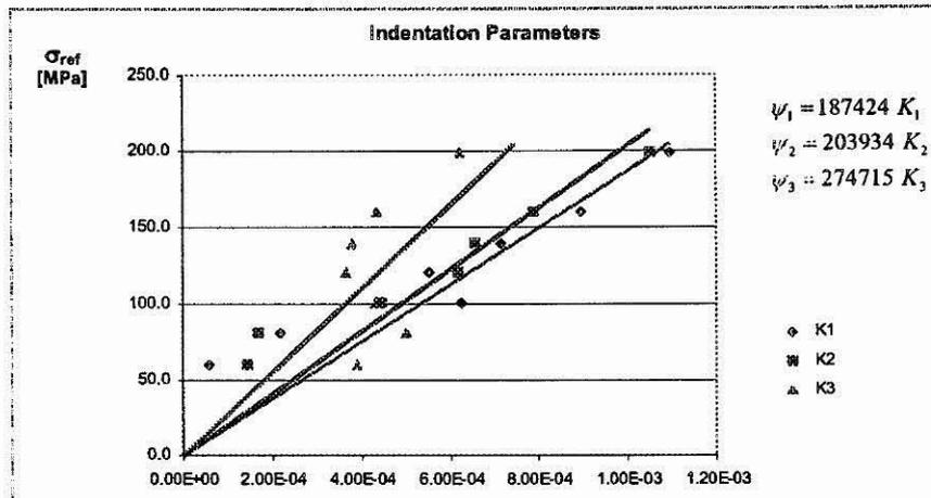
Figure 5.2 Indentation parameter versus reference residual stress.
