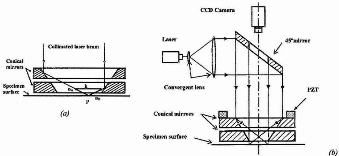
Figure 2.1 Double illumination through the radial interferometer.
