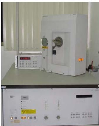
**Fig. 11 – Difratoômetro de Raios-X (Philips PW1840)**
