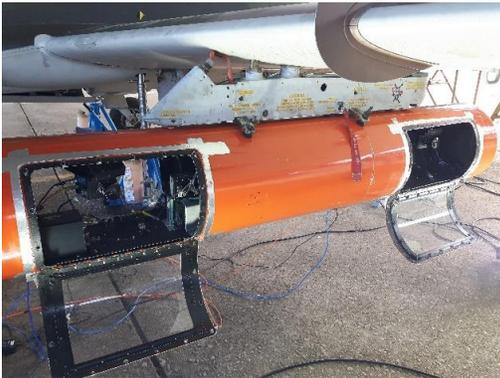
Figure 8: Camera POD installed under wing of the XAT-26 aircraft.
