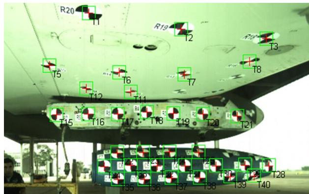
Figure 5: SisTrO RP marker detection and tracking.
