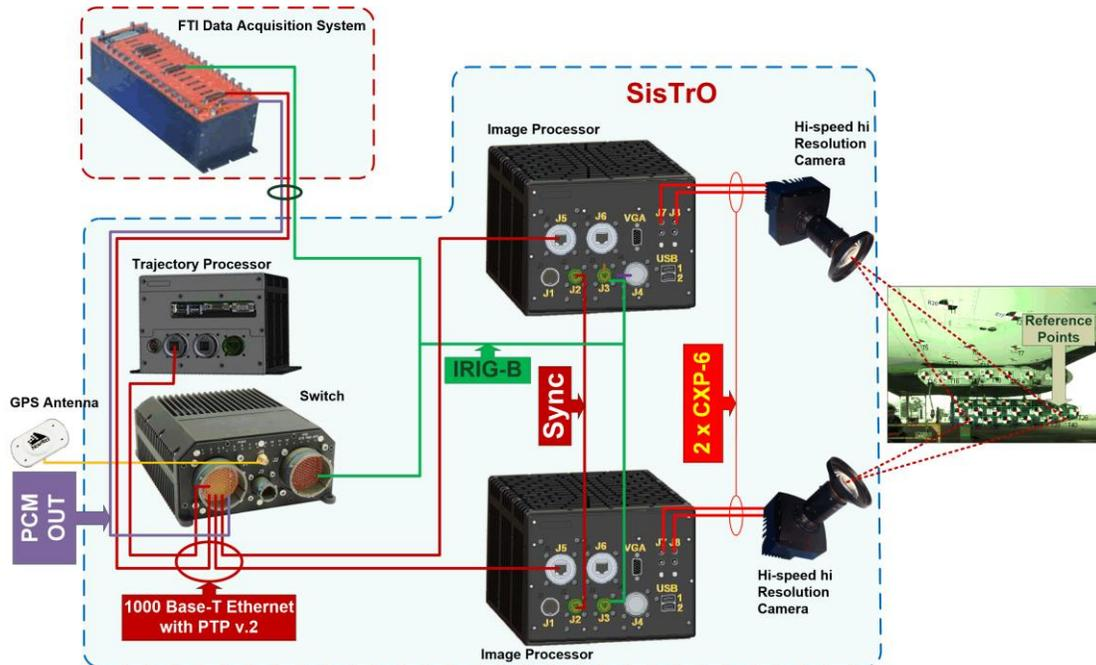
Figure 3 - SisTrO Architecture and Components.
