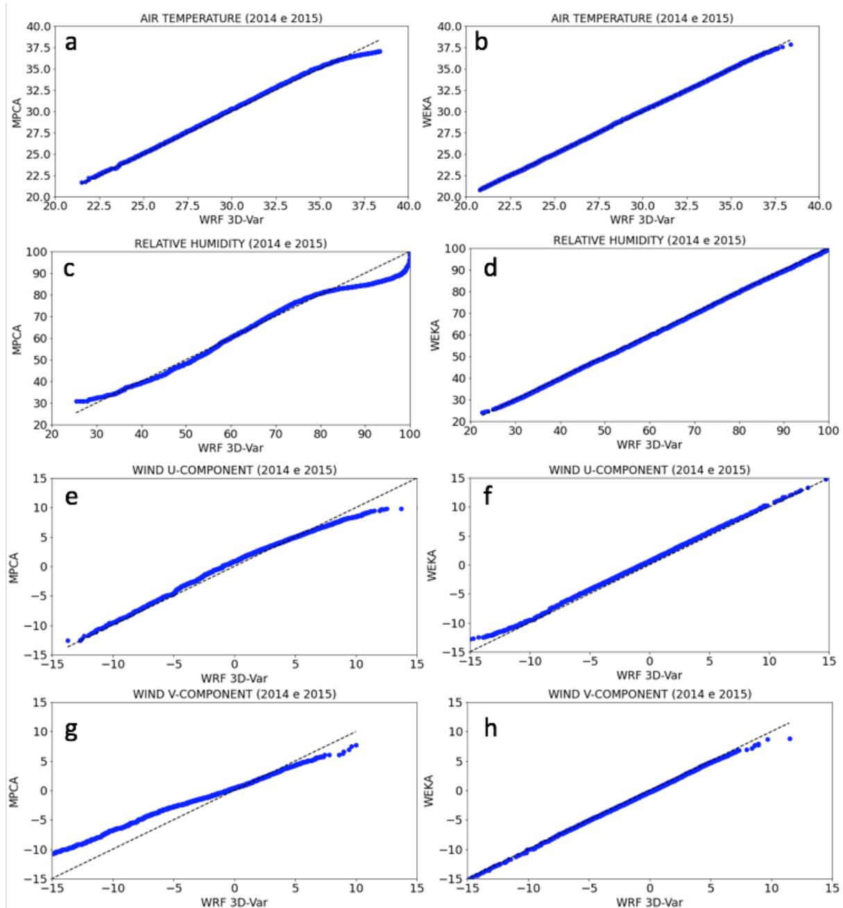
Figure 2. Quantile-quantile plot comparing the probability distribution of the trained neural networks (MPCA and Weka) (y-axis) and the actual values (x-axis) for air temperature (a and b), relative humidity (c and d), wind  $u$ -component (e and f) and wind  $v$ -component (g and h). The dashed line represents the perfect correspondence (1:1) between the trained neural network and the 3D-Var approach.
