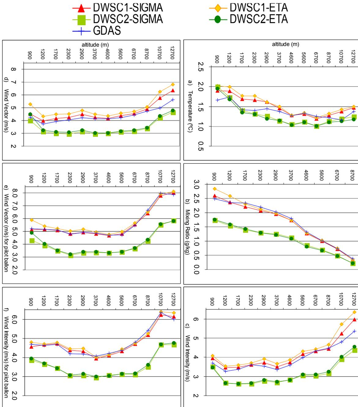
Figure 2: Variation of RMSE with altitude for a) Temperature b) Mixing Ratio c) Wind Intensity and d) Wind Vector for radiosoundings; e) Wind Vector and f) wind intensity for pilots balloons.
