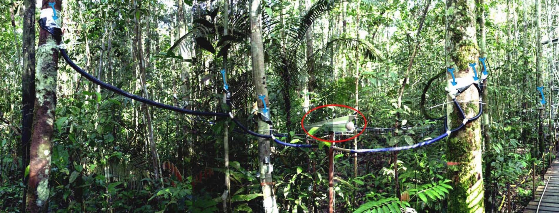
Stemflow is collected from 65 trees, using encircling-aluminum/asphalt tape shaped to divert the flow to a pipe system that join all the flows into two tipping-bucket gauges.
