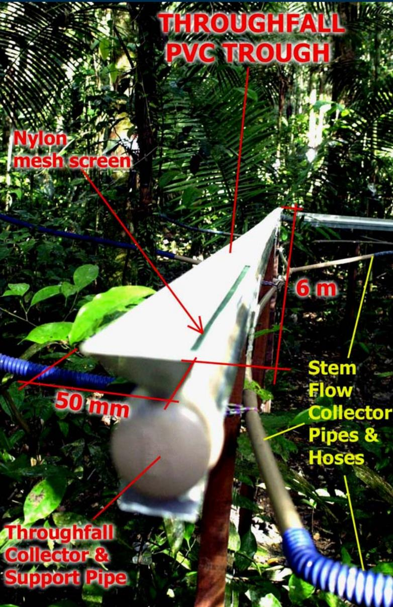
Throughfall is gauged using two sets of 5cm x 36 m V shaped troughs, connected each to a large volume tipping-bucket (125ml).
