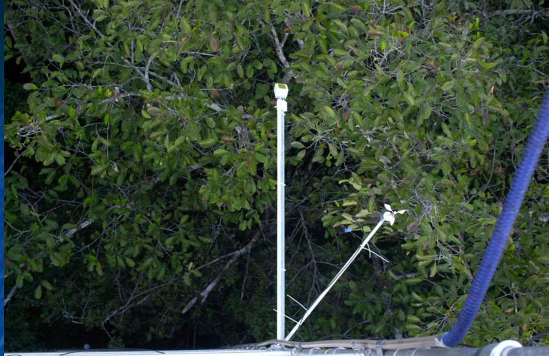
Three surface wetness logging sensors are installed offset from the towers at three heights:
