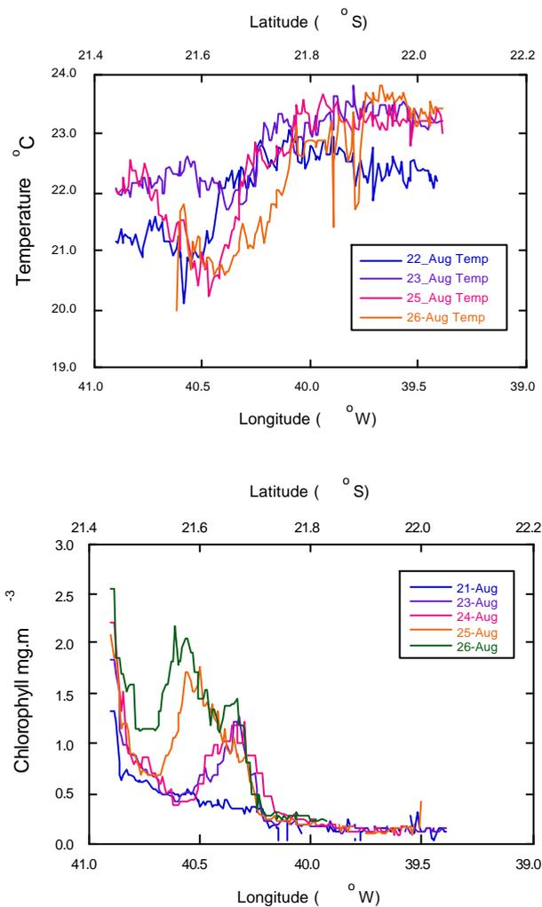
Figure 3 – SST (above) and chl (below) profiles extracted from the AVHRR and SeaWiFS satellite images, respectively.
