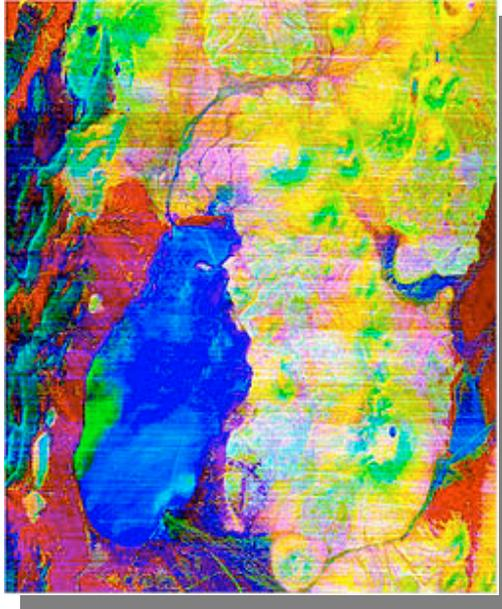
The image pair below covers a part of the White Tank Mountains of Arizona. The left image is made from 3 TIMS bands; the right is a false color composite formed from visible band data on another multispectral scanner onboard the aircraft that gathered TIMS emitted radiation.
