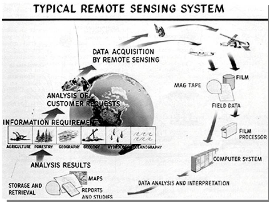
This chart shows a simple closed-loop cyclic process, unencumbered by the various feedback loops that no doubt exist. The starting point, and end point as well, is the set of panels labeled Information
