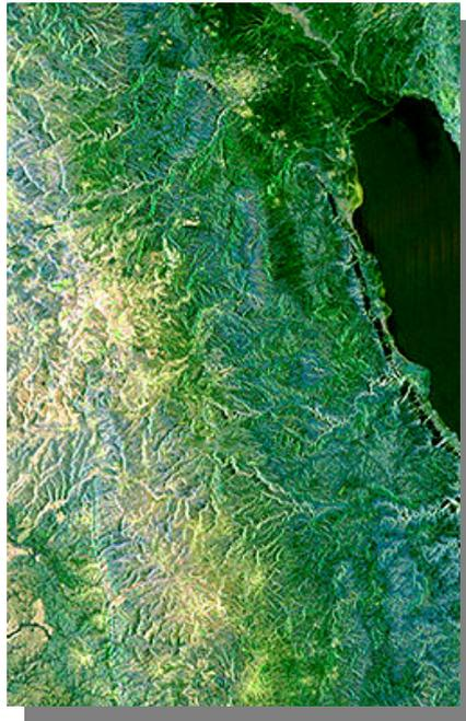
Remote sensors that cover two **thermal intervals** - the 3-5  $\mu\text{m}$  and 8-14  $\mu\text{m}$  broad bands (corresponding to two atmospheric windows) allowing sensing of thermal emissions from the land, water, ice and the atmosphere - have been flown on airplanes for several decades. Many of the meteorological satellites include at least one thermal channel. A thermal band is included on the Landsat Thematic Mapper.
