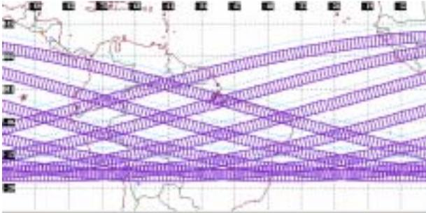
Figure 1 Coverage from an Orbit Inclined at 15°
