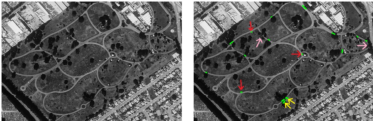
Figure 5: (a) Input image (b) The detected occlusions in green patches. The true positives are not marked with any arrow. The true negatives are marked with pink arrow. The false positives are marked with red and yellow arrows.
