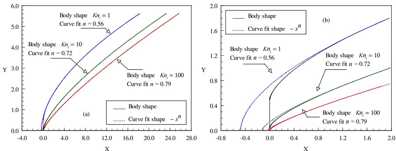
Figure 6: Comparison of flat-nose shapes with power-law curve fit shapes for leading edge thicknesses  $t/\lambda_\infty$  of 0.01, 0.1 and 1, which correspond to Knudsen number  $Kn_t$  100, 10 and 1, (a) along the afterbody surface and (b) in the vicinity of the nose.
