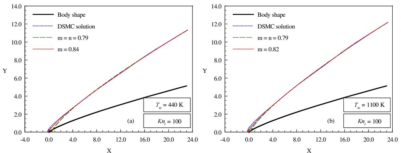
Figure 7: Shock wave shape curve fits on flat-nose body with thicknesses  $t/\lambda_\infty$  of 0.01, which corresponds to Knudsen number  $Kn_t$  100. For wall temperatures of (a) 440 K and (b) 1100 K.
