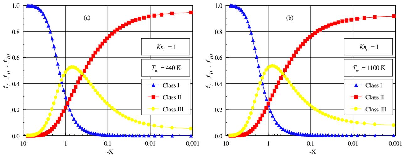
Figure 4: Distributions of molecules for classes I, II and III along the stagnation streamline for leading edge thickness that correspond to Knudsen number  $Kn_l$  of 1 and wall temperature of (a) 440 K and (b) 1100 K.
