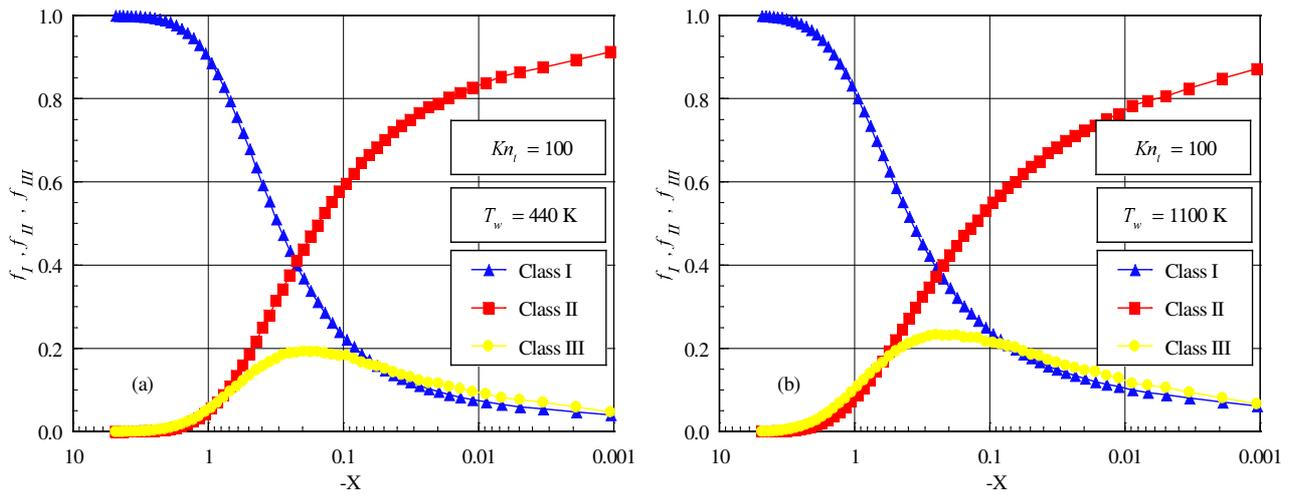
Figure 3: Distributions of molecules for classes I, II and III along the stagnation streamline for leading edge thickness that correspond to Knudsen number  $Kn_l$  of 100 and wall temperature of (a) 440 K and (b) 1100 K.
