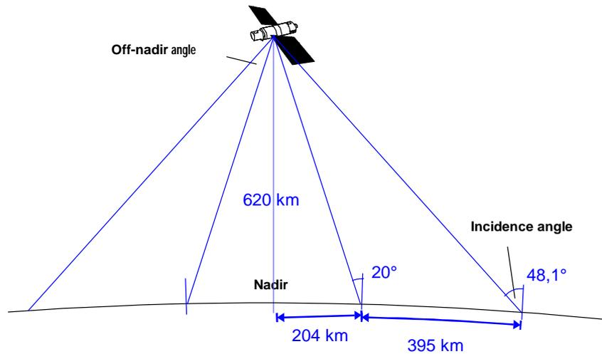
**Figure 4:** Access region of the SAR sensor.
