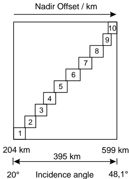
**Table 3: Radar beam specification (medium/low resolution)**
