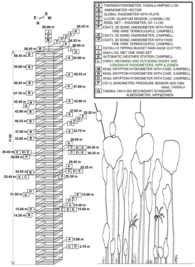
Fig 1. Schematic drawing of the micrometeorological tower located at Jaru Biological Reserve (Rebio-Jaru), with all instrumetation installed during the AMC/LBA wet season campaign
