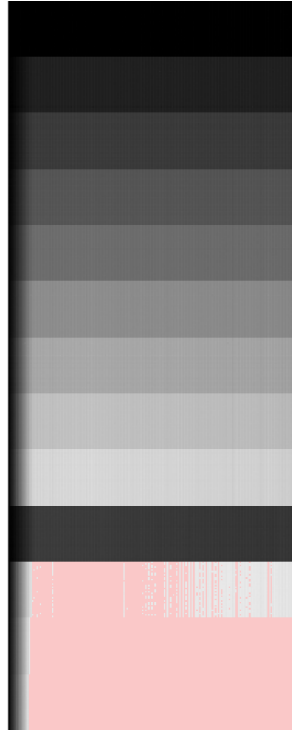
Figure 1.5.4– Calibration image for banda 2, array 1, configuration gain=1 (pink color means saturated DN values).
