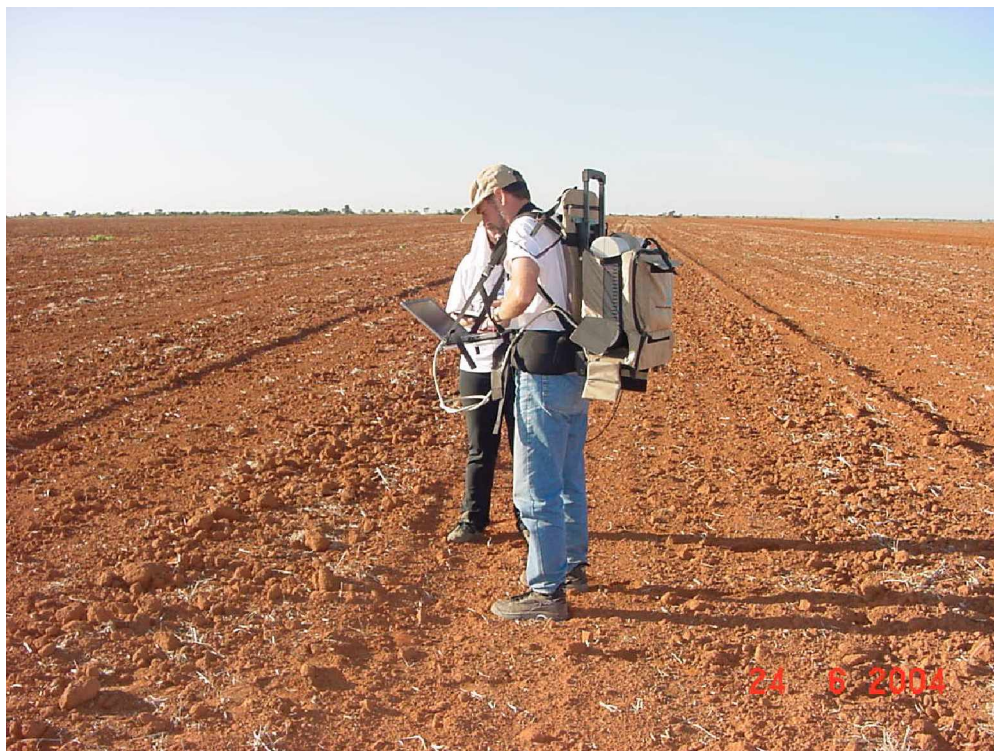
Figure 1.6.3 – Radiometric measurements performed with ASD FieldSpec spectro-radiometer in the reference surface 1.
