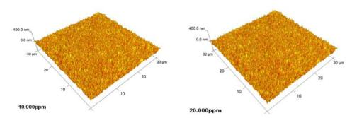
Figure 3 – Atomic Force Microscopy of the samples of BDUND1 and BDUND2.
