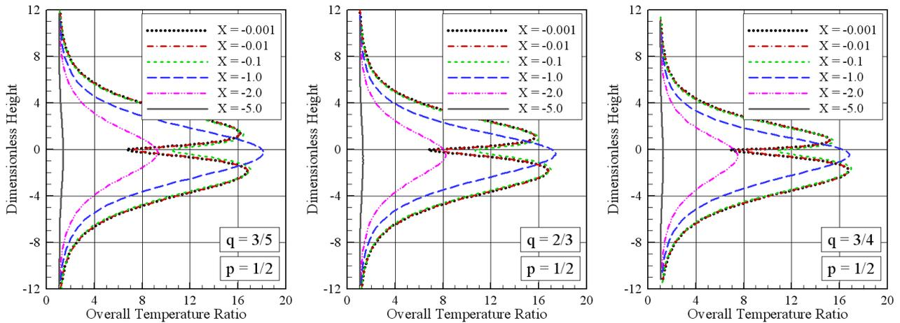
Figure 13: Overall kinetic temperature ( $T_{OV}/T_{\infty}$ ) ratio profiles upstream of the power-law leading edges corresponding to lower-surface shape of  $p = 1/2$  and upper-surface shape  $q$  of (a)  $3/5$ , (b)  $2/3$  and (c)  $3/4$ .
