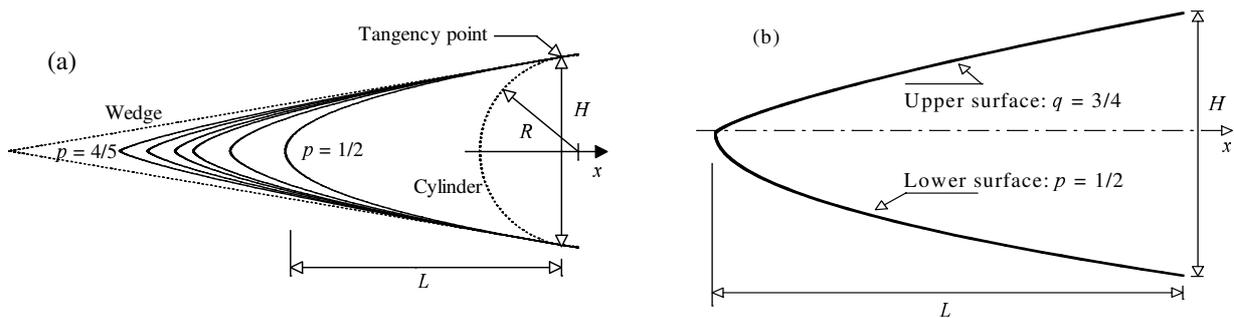
Figure 1: Drawing illustrating the (a) symmetric and (b) the asymmetric power-law leading edges.
