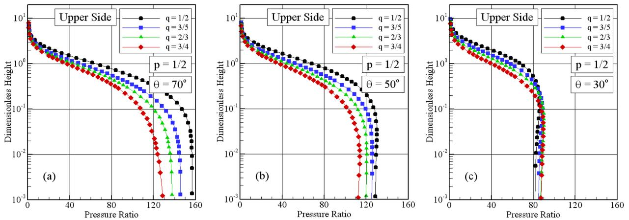
Figure 10: Pressure ( $p/p_\infty$ ) ratio profiles along the body upper surface as a function of the power-law exponent at stations corresponding to body slope angle of (a)  $70^\circ$ , (b)  $50^\circ$  and (c)  $30^\circ$  degrees.
