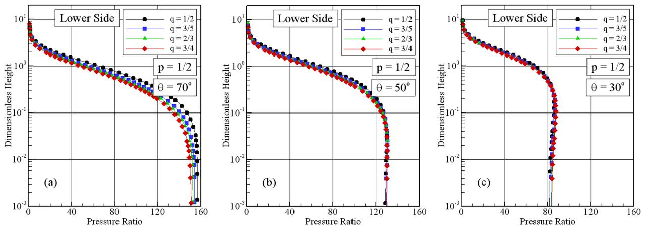
Figure 11: Pressure ( $p/p_\infty$ ) ratio profiles along the body lower surface as a function of the power-law exponent at stations corresponding to body slope angle of (a)  $70^\circ$ , (b)  $50^\circ$  and (c)  $30^\circ$  degrees.
