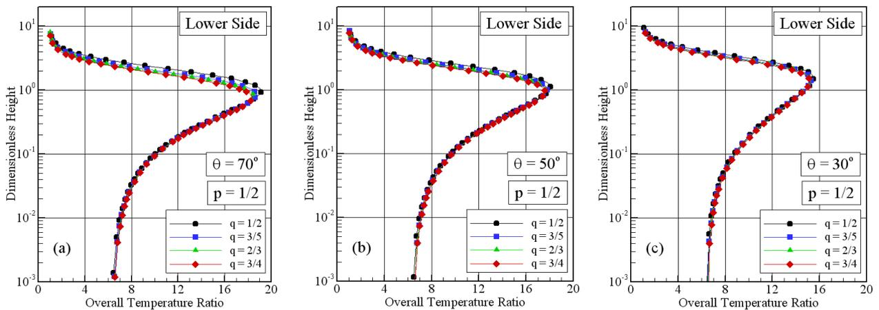
Figure 15: Overall kinetic temperature ( $T_{OV}/T_{\infty}$ ) ratio profiles along the body lower surface as a function of the power-law exponent at stations corresponding to body slope angle of (a)  $70^\circ$ , (b)  $50^\circ$  and (c)  $30^\circ$  degrees.
