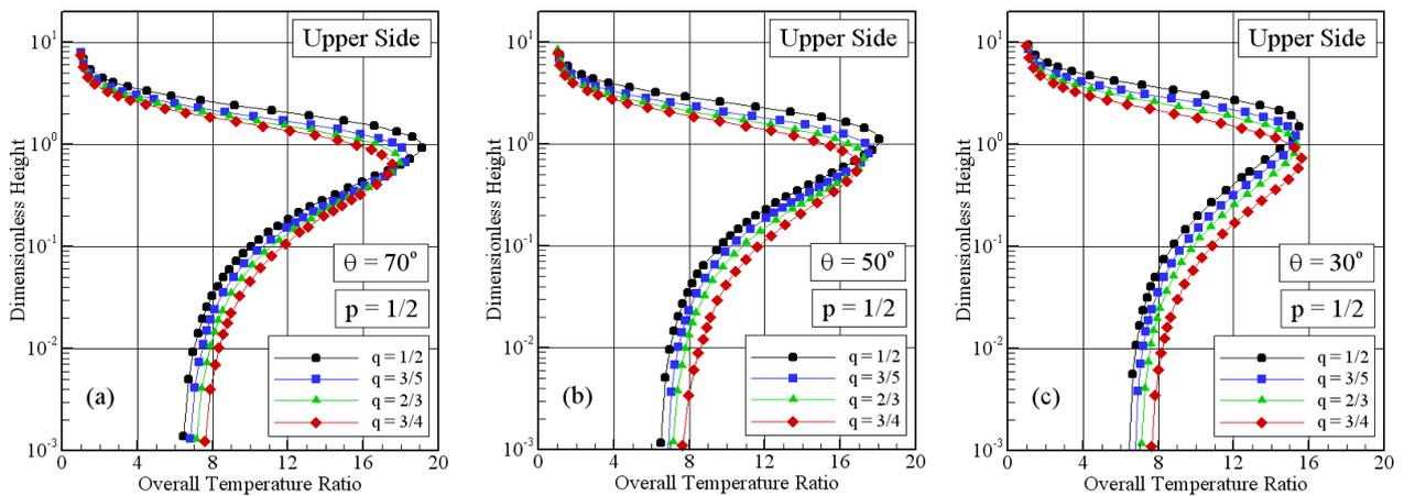
Figure 14: Overall kinetic temperature ( $T_{OV}/T_{\infty}$ ) ratio profiles along the body upper surface as a function of the power-law exponent at stations corresponding to body slope angle of (a)  $70^\circ$ , (b)  $50^\circ$  and (c)  $30^\circ$  degrees.
