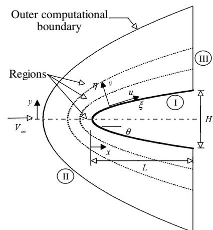
Figure 2: Drawing illustrating the computational domain.
