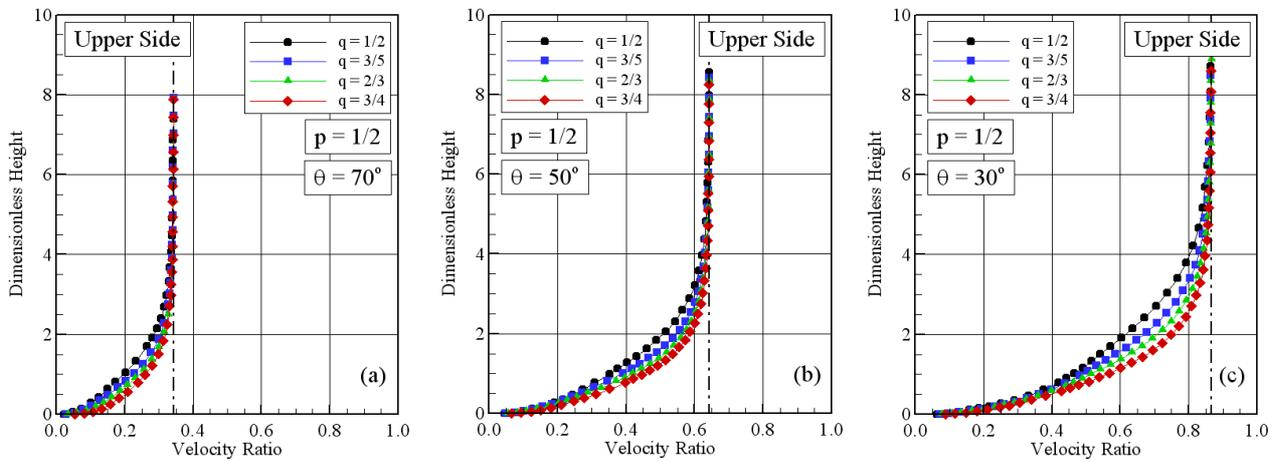
Figure 4: Tangential velocity ( $u/V_\infty$ ) profiles along the body upper surface as a function of the power-law exponent at stations corresponding to body slope angle of (a) 70, (b) 50 and (c) 30 degrees.
