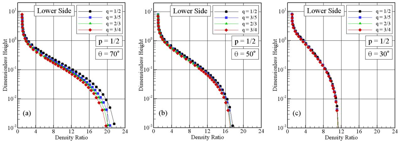
Figure 8: Density ( $\rho/\rho_\infty$ ) ratio profiles along the body lower surface as a function of the power-law exponent at stations corresponding to body slope angle of (a) 70, (b) 50 and (c) 30 degrees.
