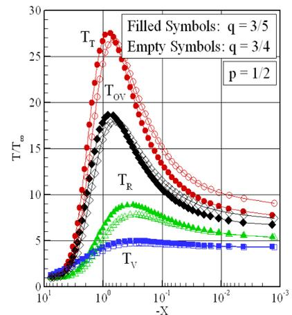
Figure 12: Kinetic temperature ( $T/T_\infty$ ) profiles along the stagnation streamline as a function of the power-law exponent  $q$ .
