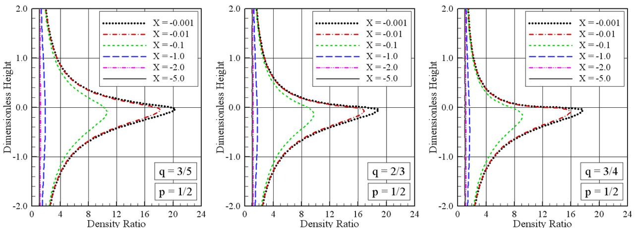
**Figure 6: Density ( $\rho/\rho_\infty$ ) ratio profiles upstream of the power-law leading edges corresponding to lower-surface shape of  $p = 1/2$  and upper-surface shape  $q$  of (a) 3/5, (b) 2/3 and (c) 3/4.**
