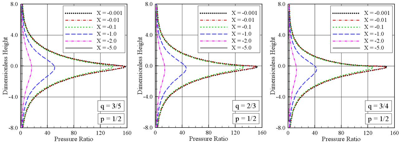
Figure 9: Pressure ( $p/p_\infty$ ) ratio profiles upstream of the power-law leading edges corresponding to lower-surface shape of  $p = 1/2$  and upper-surface shape  $q$  of (a)  $3/5$ , (b)  $2/3$  and (c)  $3/4$ .
