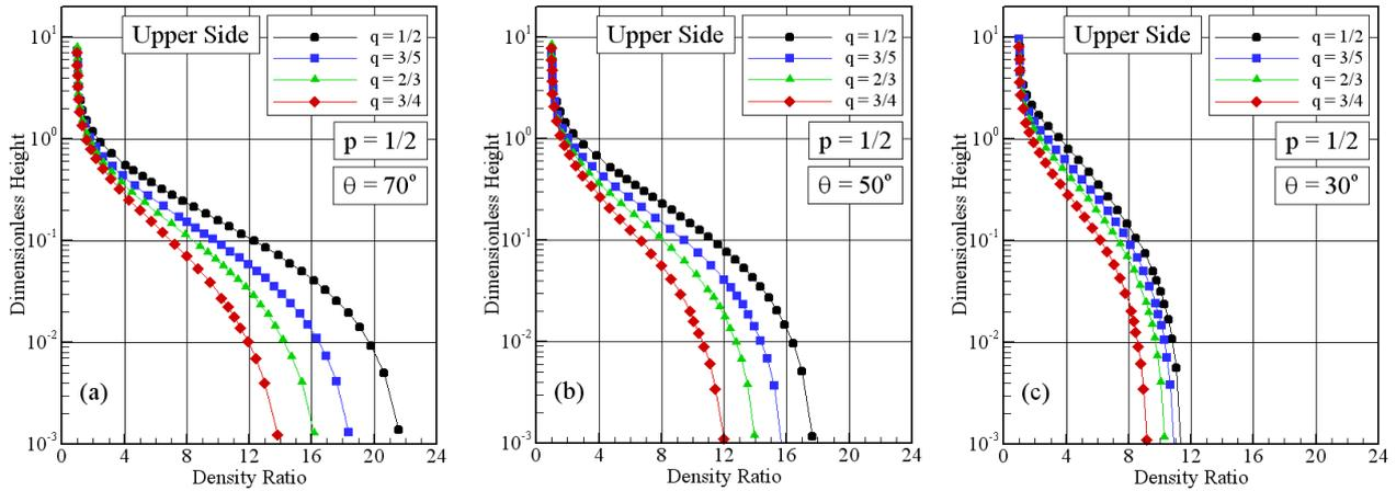
Figure 7: Density ( $\rho/\rho_\infty$ ) ratio profiles along the body upper surface as a function of the power-law exponent at stations corresponding to body slope angle of (a) 70, (b) 50 and (c) 30 degrees.
