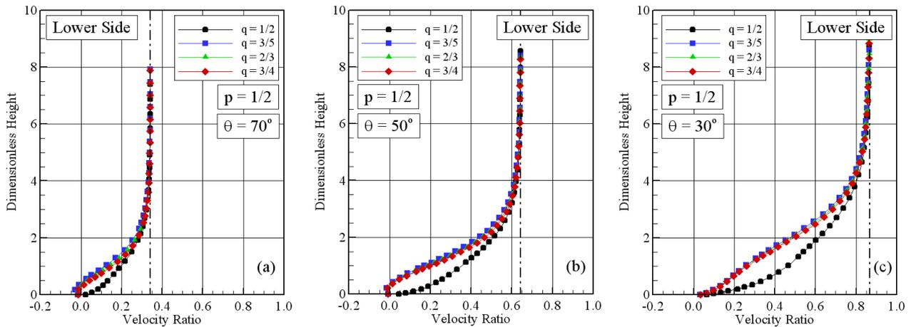
Figure 5: Tangential velocity ( $u/V_\infty$ ) profiles along the body lower surface as a function of the power-law exponent at stations corresponding to body slope angle of (a) 70, (b) 50 and (c) 30 degrees.
