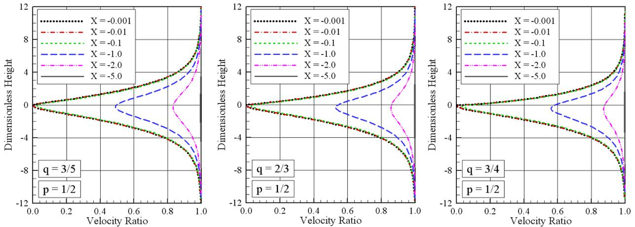
Figure 3: Normal velocity ( $v/V_\infty$ ) profiles upstream of the power-law leading edges corresponding to lower-surface shape of  $p = 1/2$  and upper-surface shape  $q$  of (a) 3/5, (b) 2/3 and (c) 3/4.
