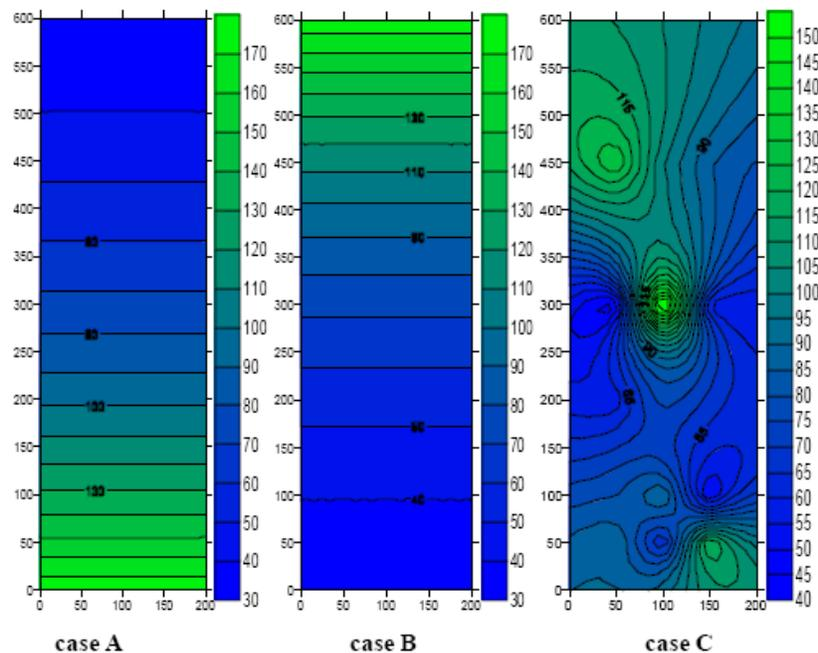
Figure 1: Contour Map of Hydraulic Conductivity for the different distribution used in the simulation experiment.
