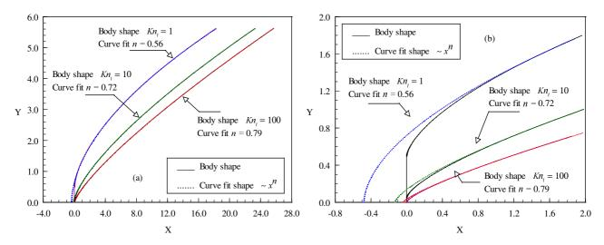
Figure 6: Comparison of flat-nose shapes with power-law curve fit shapes for leading edge thicknesses  $t/\lambda_{\infty}$  of 0.01, 0.1 and 1, which correspond to Knudsen number  $Kn_t$  100, 10 and 1. (a) along the afterbody surface and (b) in the vicinity of the nose.
