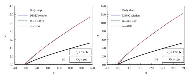
Figure 7: Shock wave shape curve fits on flat-nose body with thicknesses  $t/\lambda_{\infty}$  of 0.01, which corresponds to Knudsen number  $Kn_t$  100. For wall temperatures of (a) 440 K and (b) 1100 K.
