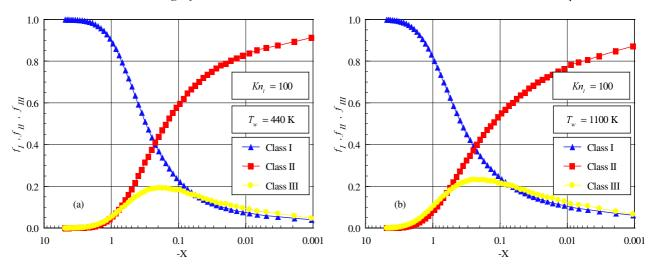
Figure 3: Distributions of molecules for classes I, II and III along the stagnation streamline for leading edge thickness that correspond to Knudsen number  $Kn_t$  of 100 and wall temperature of (a) 440 K and (b) 1100 K.
