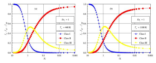
Figure 4: Distributions of molecules for classes I, II and III along the stagnation streamline for leading edge thickness that correspond to Knudsen number  $Kn_t$  of 1 and wall temperature of (a) 440 K and (b) 1100 K.
