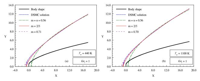
Figure 8: Shock wave shape curve fits on flat-nose body with thicknesses  $t/\lambda_{\infty}$  of 1, which corresponds to Knudsen number  $Kn_t$  1. For wall temperatures of (a) 440 K and (b) 1100 K.
