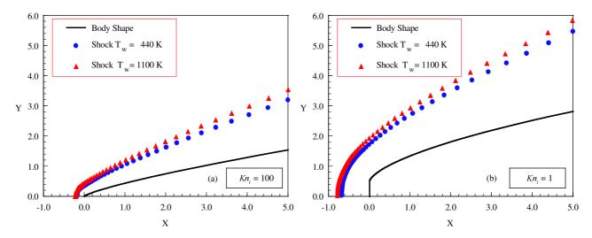
Figure 5: Shock wave shapes on flat-nose bodies as a function of the wall temperature for leading edge thicknesses that correspond to Knudsen number  $Kn_t$  of (a) 100 and (b) 1.
