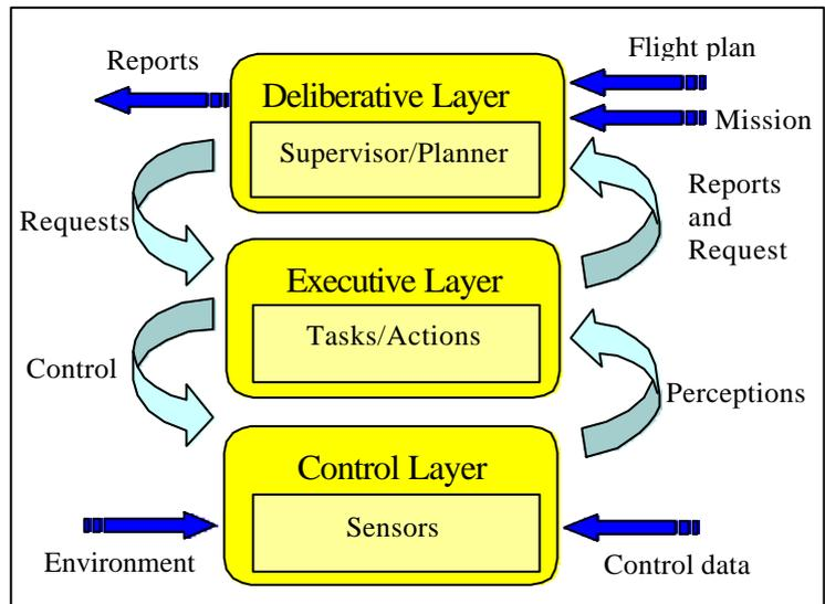
**Figure 4** – Robotic software architecture
