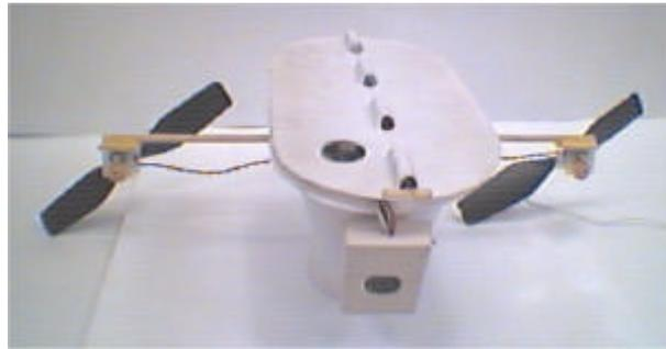
**Figure 2** – The gondola and the CCD camera
