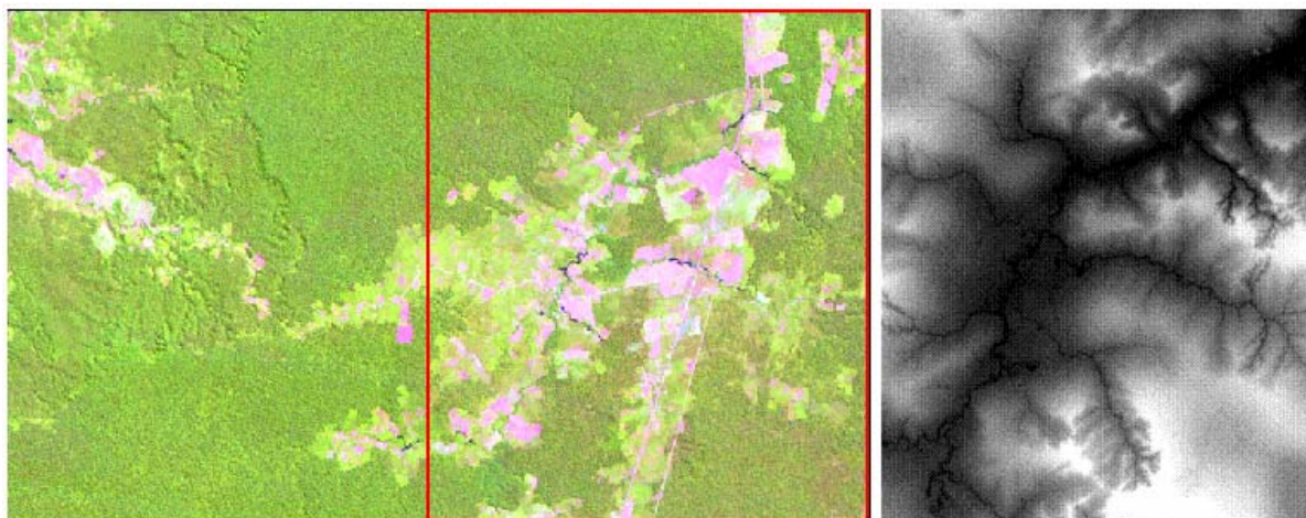
Figure 1 - TM LANDSAT/5 RGB-543 (left side). The red rectangle corresponds to P band InSAR DEM area (right side).
