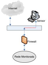
Figure 2: Network sensor placing in the monitored network
