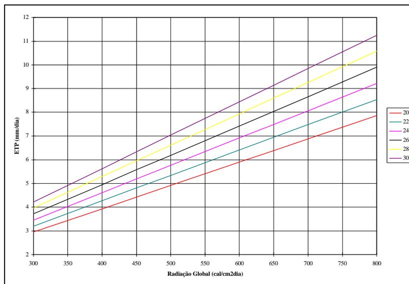
Figure 3 - Variation of the ETP with global solar radiation for different air temperature using MJH method.
