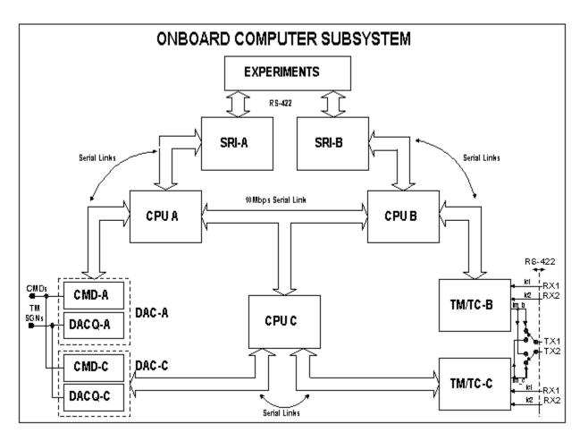
Fig. 3: On-board Computer Subsystem Block Diagram.
