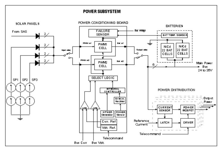
Fig. 2: Power Supply Subsystem Block Diagram SACI-1
