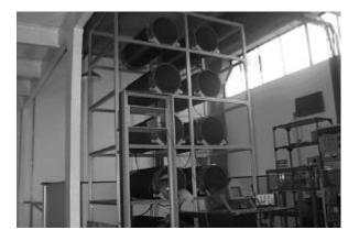
Fig. 1. The pulse generator structure.
