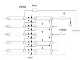
Fig. 1. A coaxial Blumlein pulser made of 10 lines.
