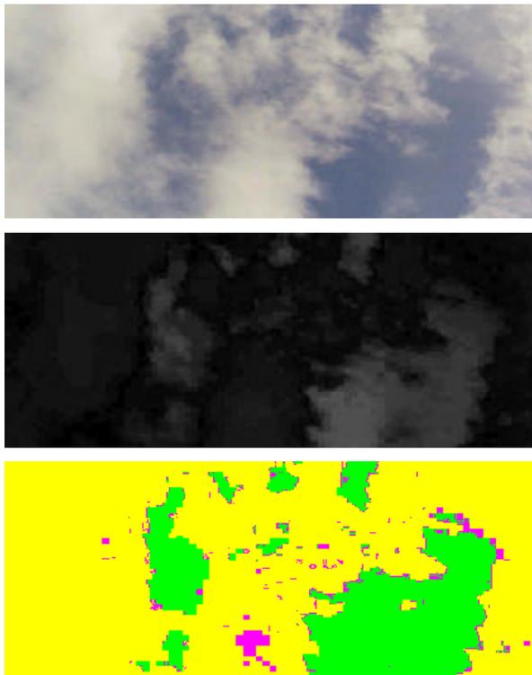
Figure 5. From top to bottom, these illustration depicts, (a) the original CCD image in RGB, (b) the mage of pixel saturation, and (c) map of false colors generate by the algorithm.
