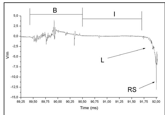
Figure 2 – An example of the type of the electric field waveform analyzed in this paper. In this figure the three stages B, I and L are clearly observed.
