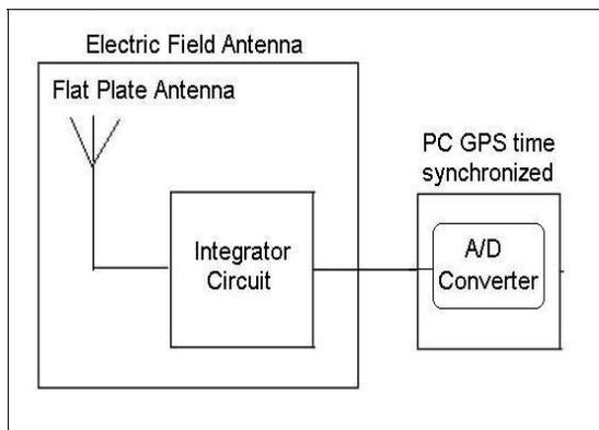
Figure 1 – Electric field acquisition apparatus used to obtain the data analyzed in this work.
