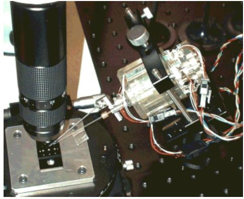
Dimensions: cylindrical hand 48mm outer diameter, 65mm high (3 internal PZT actuators are used for each finger) Working range: approx. 100 x 100 x  $30\mu$ m Resolution of motion:  $1\mu$ m or less Object motion control:  $200\mu$ m max.
