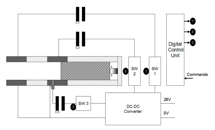
Figure 3 – A block diagram of the HFB-PPT.
