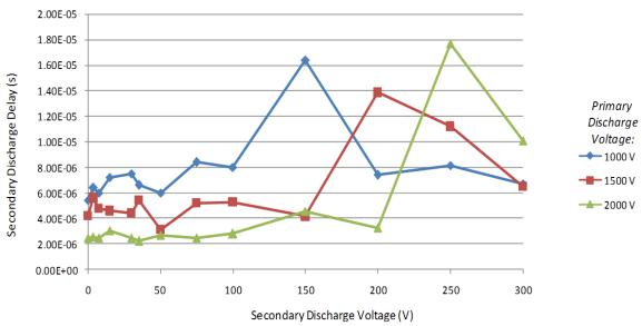
Figure 9. – Delay between the first discharge and the second discharge as a function of the voltage applied to the secondary electrodes for three different primary discharge voltages.
