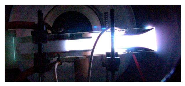
Figure 11. – HFB-PPT firing.
