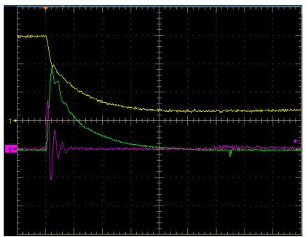
Figure 7. – Fourth regimen. Typical discharge for secondary discharge voltages above 150 V (for 1 kV main discharge), 200 V (for 1.5 kV main discharge) or 250 V (for 2 kV main discharge), showing the secondary discharge capacitor voltage (yellow, 100V/div), secondary discharge current (green, 1000 A/div) and primary discharge current (pink, 5000 A/div) at 100 µs/div (horizontally). Taken with 1.5kV primary discharge and 300 V secondary discharge.
