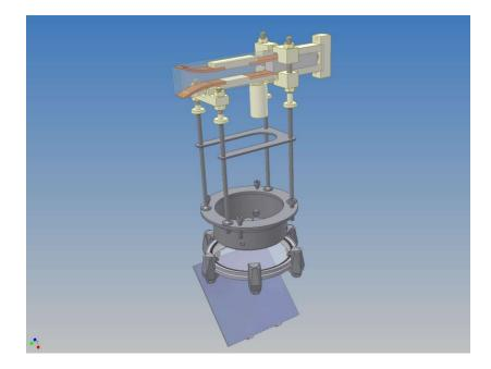
Figure 2 - The model of the developed HFB-PPT (top) mounted on its support (center) with a mirror on the bottom for instrumentation purposes.
