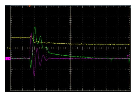
Figure 6. – Third regimen. Typical discharge for secondary discharge voltage between 75 V and 100V (for all three primary voltages), showing the secondary discharge capacitor voltage (yellow, 100V/div), secondary discharge current (green, 500 A/div) and primary discharge current (pink, 5000 A/div) at 100  $\mu$ s/div (horizontally). Taken with 2kV primary discharge and 100 V secondary discharge.
