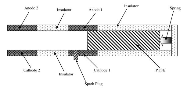
Figure 1 – HFB-PPT Discharge Chamber.
