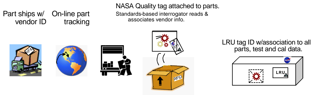
Figure 3-3: RFID Ground-to-Line Replacement Unit Concept
