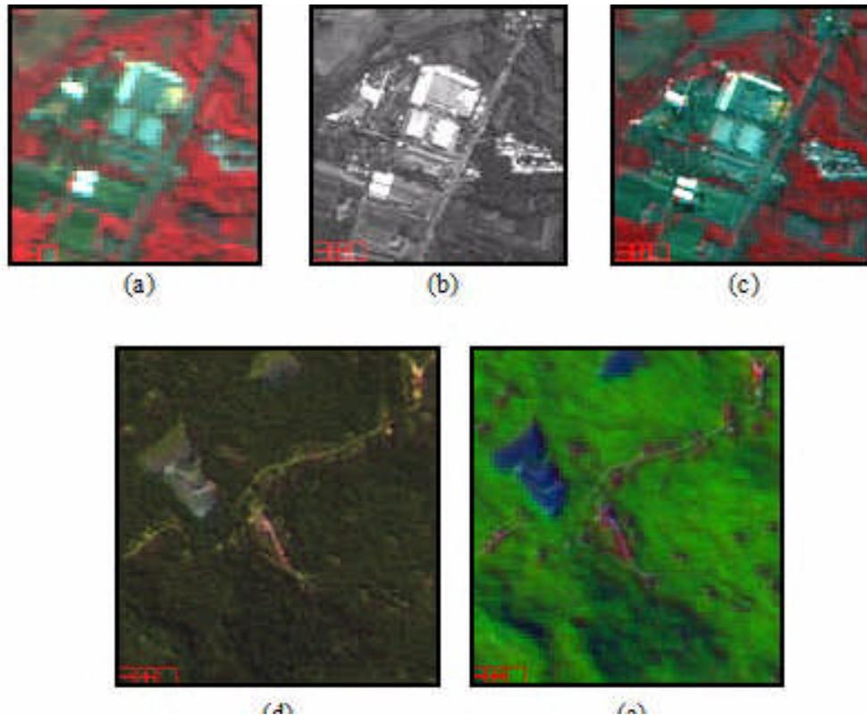
Figure 4.2 Multispectral SPOT Image 10 m (a) Panchromatic SPOT 2.5 m (b) Pan-sharp Multispectral SPOT 2.5 m (c) HIS Pan-sharpening (d) Gram-Schmidt Pan-sharpening (e)
