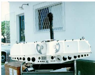
Fig.1 – Espectrofotômetro Dobson (INPE – CRN)
