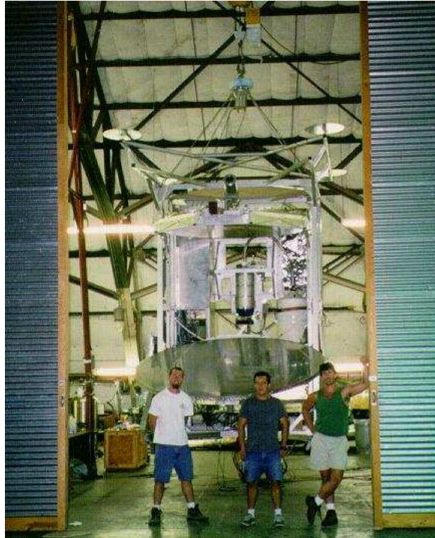
Fig. 8 - BEAST in its dome in White Mountain. The size of the instrument and components can be figured out by comparing with investigators in front of the gondola. They are about 1,80 m tall.
