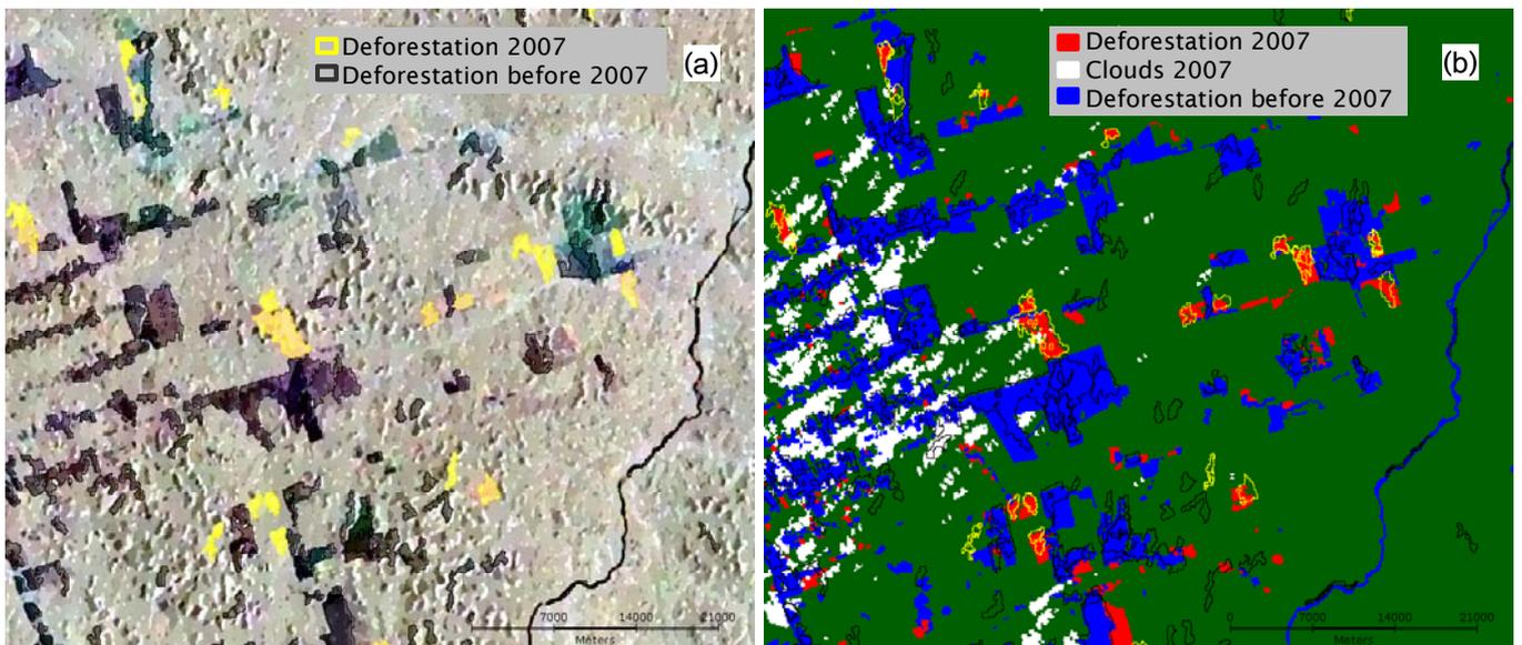
Figure 8. Deforestation polygons from ALOS PALSAR ScanSAR 2007 classification (yellow vectors) over (a) color composition 2007-08-30 (R), 2007-07-13 (G), 2007-05-28; and (b) PRODES 2008 deforestation mapping
