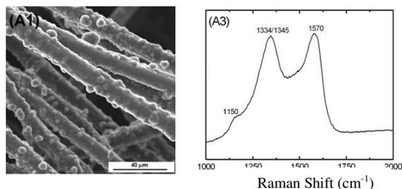
**Fig. 2.** (A1)-SEM images of ND/CF-1000. (A3)- Raman spectrum of ND covering the CF-1000
