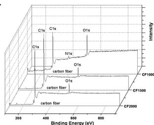
**Fig. 1.** Survey spectra of CF-1000, CF-1500 and CF-2000.
