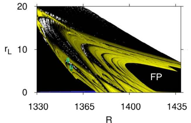
**Figure 1 – Global view of the  $(R, r_L)$  parameter space of Eqs. (1). The axes are in resistance units (Ohms). Black color indicates periodic behavior, yellow one indicates chaotic behavior. The white region indicates fixed points. The blue region indicates divergence of Eqs. (1). The black region marked with FP, is another fixed points region. The points 'a' and 'b' locate the parameter values of the attractors shown in Fig. 2.**
