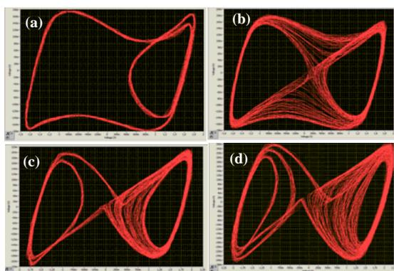
Figure 3 – Four experimental attractors for the implemented chaotic circuit. See the similarities between the attractors (a) and (b) with the theoretical attractors (a) and (b) in Fig. 2.
