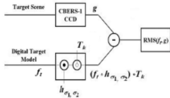
Figure 5: Block diagram of the PSF estimation.
