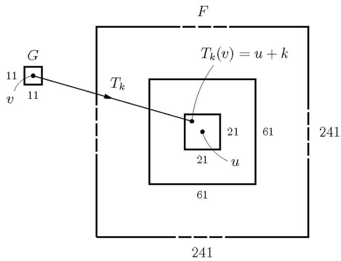
Figure 4: Digital target model (dimensions are in meter).
