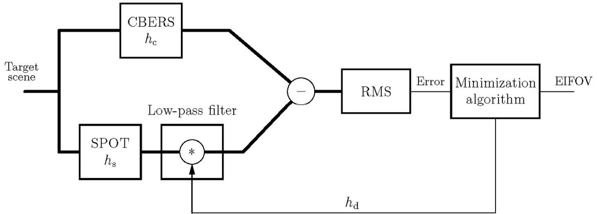
Figure 18: Block diagram of the low-resolution image simulation process.
