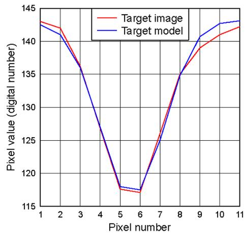
Figure 7: Across-track fitting for band 3 of CBERS-1 (pixel number versus pixel value).
