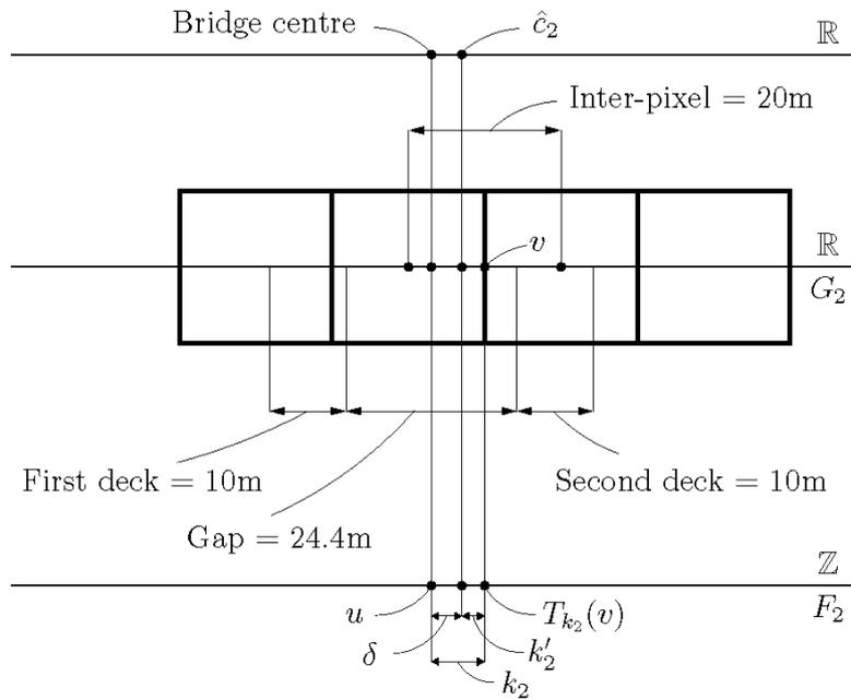
Figure 13: Causeway bridge model.
