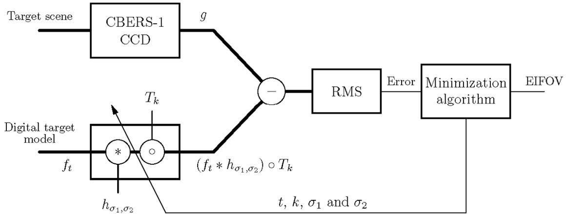
Figure 5: Block diagram of the PSF identification process.
