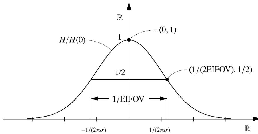
Figure 1. Relation between the EIFOV parameter and the Gaussian MTF graph.
