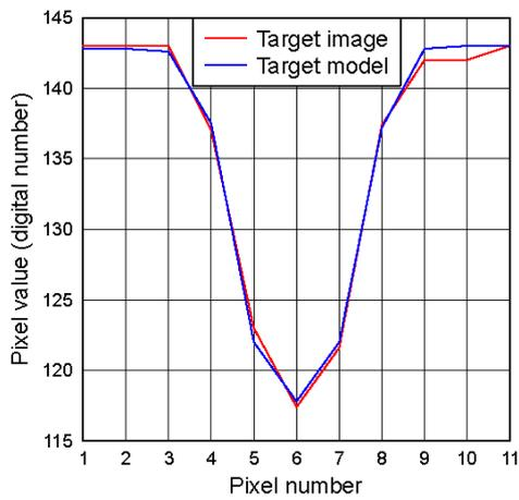
Figure 6: Along-track fitting for band 3 of CBERS-1 (pixel number versus pixel value).
