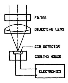
Fig. 1 - Diagram of the Imaging Spectral Photometer.
