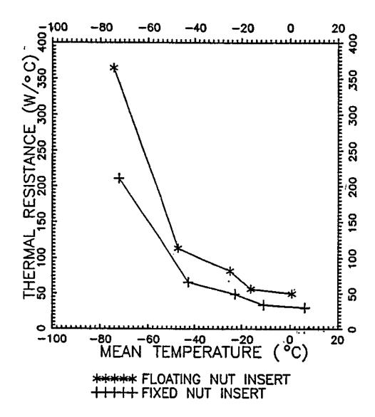
Figure 5. Thermal resistance as a mean temperature function for the two studied joints.
