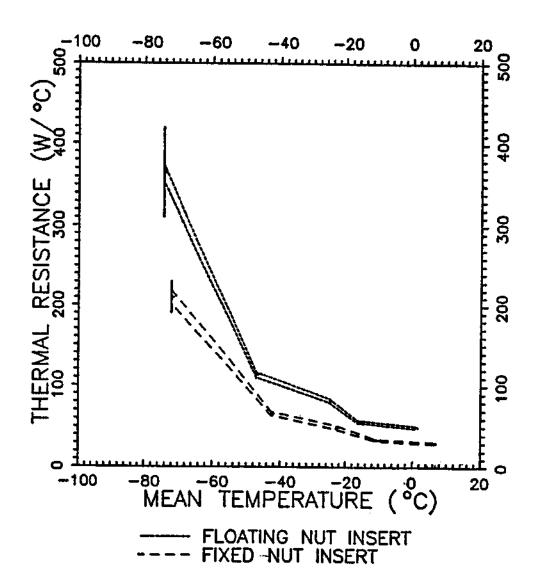
Figure 6. Thermal resistance as a mean temperature function with its associated experimental and standard errors.
