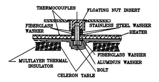
Figure 3. Floating nut insert joint experimental apparatus.
