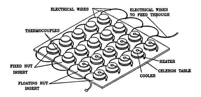
Figure 4. Final experimental mounting in Celeron table.
