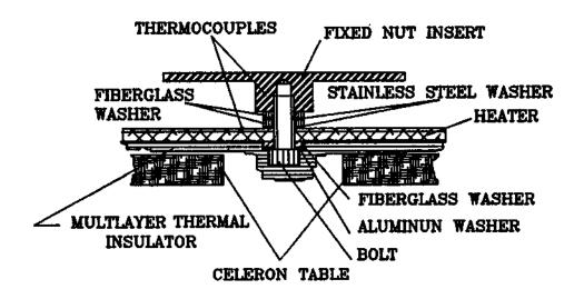
Figure 2. Fixed nut insert joint experimental apparatus.
