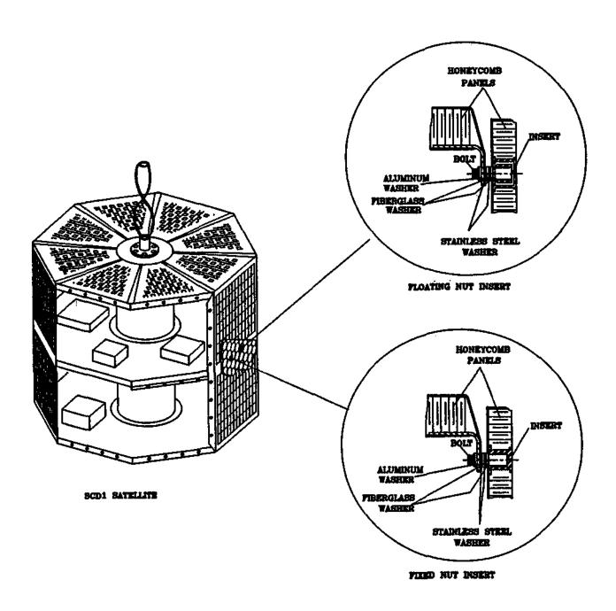
Figure 1. SCD1 schematic view, with the localization of the studied bolted joints.
