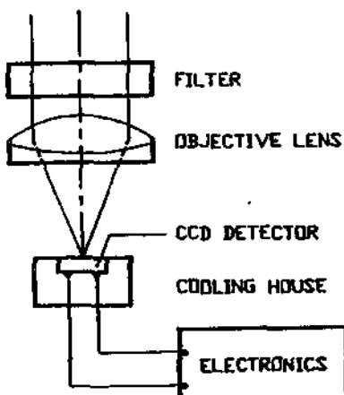
Fig. 1 - Diagram of the Imaging Spectral Photometer.
