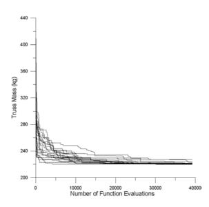
Figure 6. Best value of truss mass as a function of number of evaluations for 20 independent runs of GEO.
